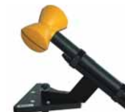
The single-axis antennas can be mounted on a tripod and adjusted to produce isotropic results by making measurements in three mutually perpendicular positions. Hand-held, they are also ideal for locating maximum values within a room using the so-called pendulum method.
