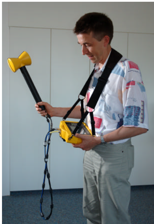
Figure 2: The Selective Radiation Meter SRM-3000 with single axis antenna and "Maximum Hold" function used for the panning method.
