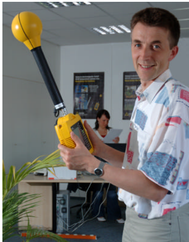
Figure 1: The Selective Radiation Meter SRM-3000 fitted with a plug-in isotropic antenna is ideal for space measurements without the need to twist or turn.
