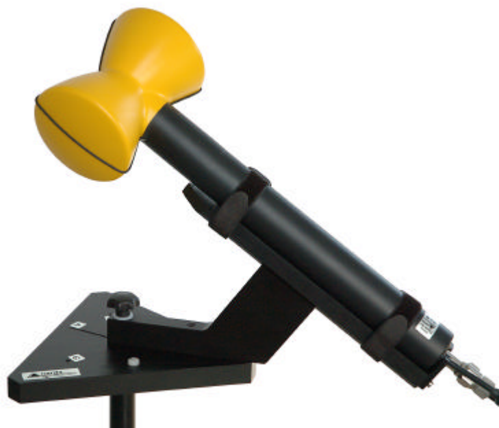
Figure 3: Single axis antenna on a rotating platform. The test instrument calculates the isotropic result automatically from three separate measurements at defined positions. Low ellipticity in the directional characteristic is essential for accuracy.
