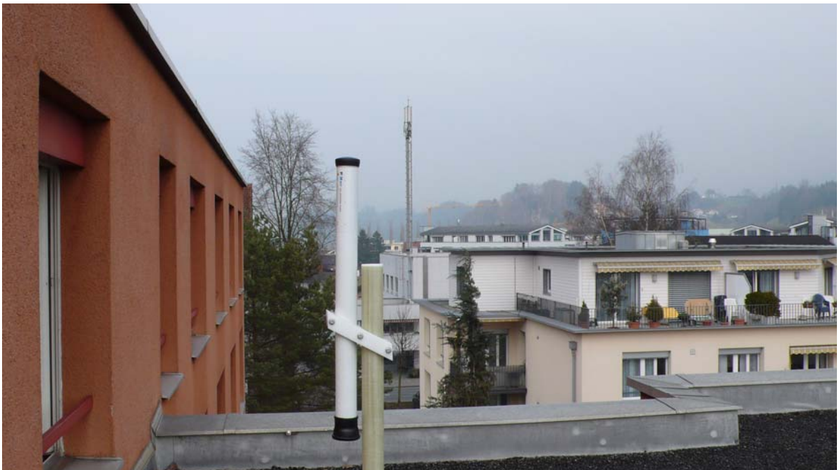
Figure 1: Measuring probe located at "Sarnen" (flat roof of a retirement home). A mobile phone transmitter mast can be seen in the background.
