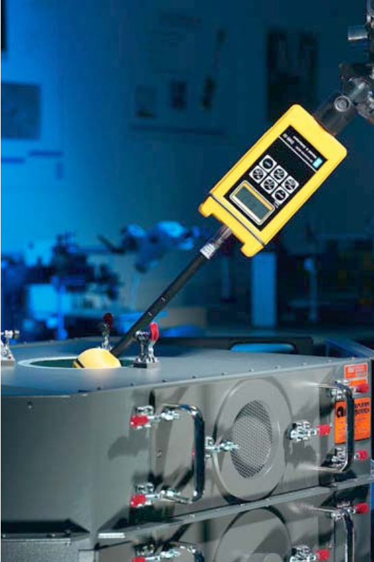
Device under test in a TEM cell (photo at the right)
