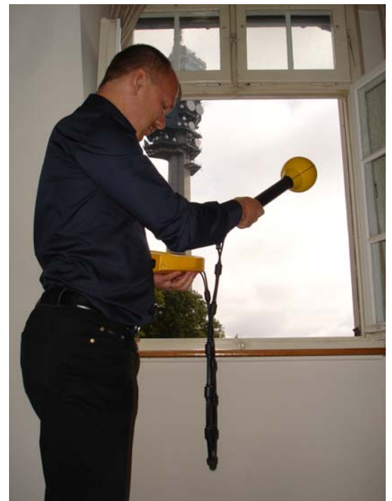
Making measurements with the SRM-3000 by the TV tower in Sankt Chrischona (Basel)
