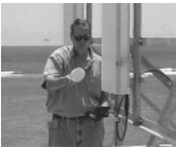
Measuring field strength in front of a directional "sector" antenna.
