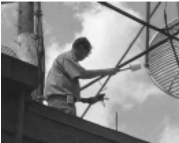
Measuring field strength near a parabolic antenna.
